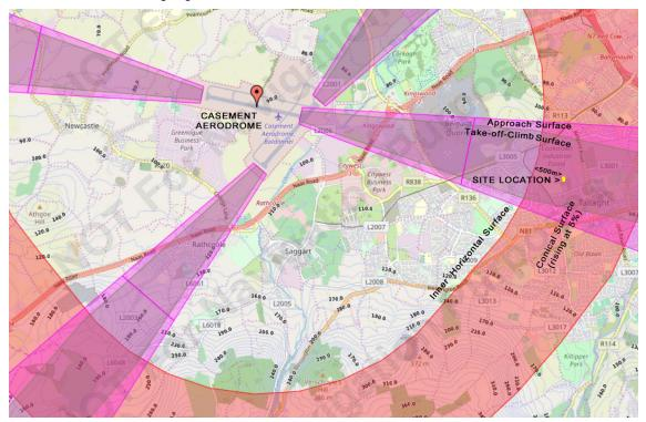
7.2 It can be seen that this site lies under the Conical Surface of Casement Aerodrome (as well as being under – but not projecting above – the Approach and Take-Off-Climb Surfaces to/from Runways 10/28). The Conical Surface (although much less important at an aerodrome than the more critical Approach and Take-Off Climb Surfaces) is, in this location, the lowest of the three Obstacle Limitation Surfaces which affect this site.
