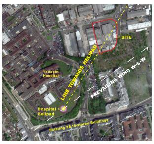
The building layout on the site has been designed to render its shape more suited to helicopter movements to/from the nearby helipad: i.e. with lower building height towards the corner nearest the helipad, and with height increasing from south to north, towards the corner farthest from the helipad – so that all of the building will lie below a 1 in 8 slope leading to the edge of the helipad (in accordance with the international guidelines described in §10.4 & §10.5 below).
