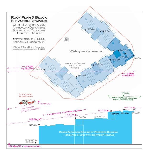
10.5 It can be seen from the Plan & Block Elev. drawing above that the proposed building, which steps down towards the helipad site,
